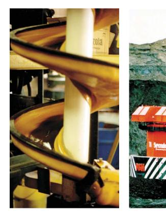
Spirals separate different density minerals using centrifugal force (left). Oil sand mining uses large-scale shovels and trucks (right)
